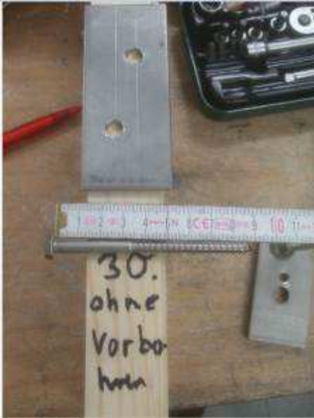
Picture 3 6.0x90 Din 571 without pre-drilling
