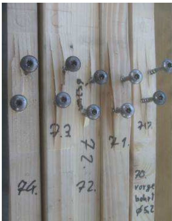
Picture 22 Breakage picture of the pulled out screws
