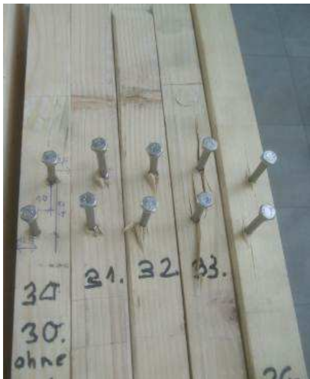
Picture 14 Failure picture of the pulled out screws
