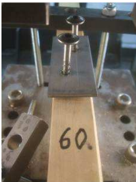
Picture 9 8.0 x 100 wafer-head screw Screwed down to a depth of 60 mm
