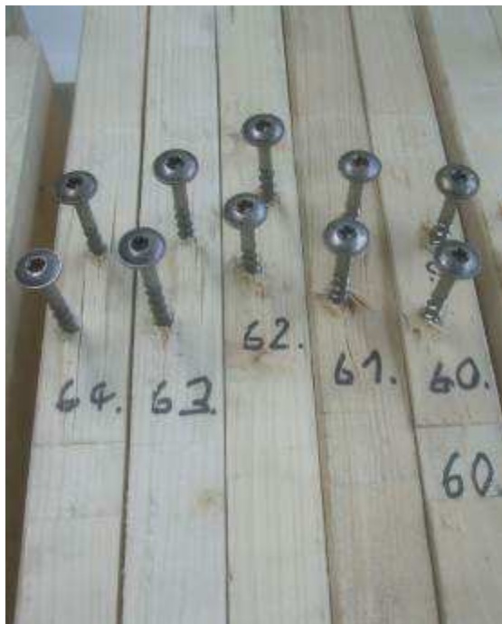
Picture 20 Breakage picture of the pulled out screws
