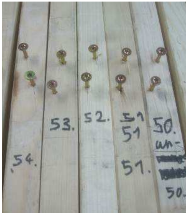
Picture 18 Breakage picture of the pulled out screws
