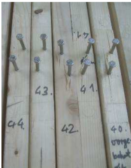
Picture 16 Breakage picture of the pulled out screws
